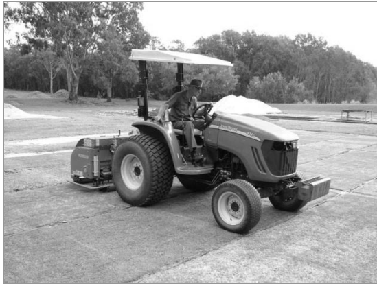
FIGURE 3 (a) Decompaction treatments being imposed to D1 and D6 plots on 15 Jun 2009 at RRF by Terry Griffiths of Q Turf Machinery; (b) Verti-Drain decompaction unit using 20 mm solid tynes; and (c) impact of decompaction treatment on worn plots showing 150 mm spacings.
